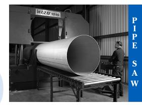
RJS boasts one of the country's largest pipe saws, capable of handling up to 36" pipe.
